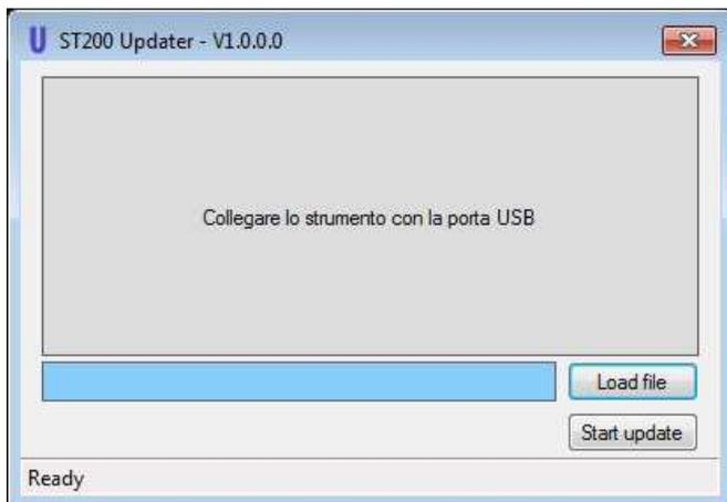
5- Connect the PC to the instrument by using a USB cable supplied and select **“Load file”**
