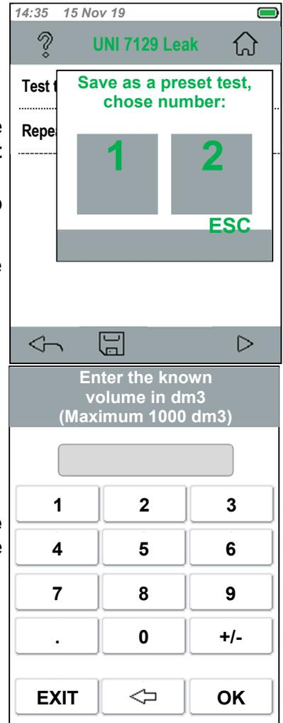
If the **Manual** method has been selected in the **System volume** parameters or in **Pressurizing**, a screen will appear, where the value can be entered by using the touch keyboard.
