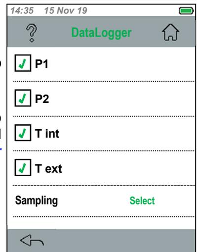
After selecting the Values to be recorded and the Sampling Time, the recording is started by pressing
