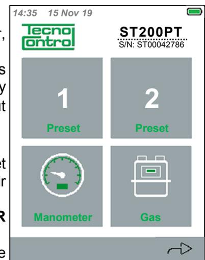
This page contains 4 additional keys to manage the data associated with the **REGISTRY**, **ARCHIVE**, **DATALOGGER** and, lastly, the instrument **SETTINGS** (See the relevant chapters that follow).
