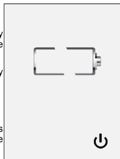
When the lithium battery is fully charged, the display graphically shows that the battery has reached its maximum charge.
