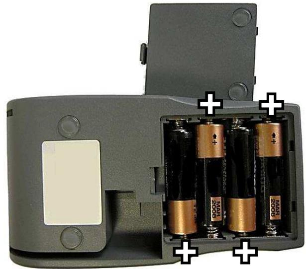
**i** For a longer printing time, we recommend using good quality alkaline batteries.
